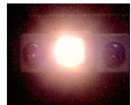
Prototype of white LED warm white type (correlated color temperature 2,800K)
