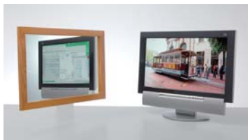
Two-way viewing-angle LCD (prototype) One user sees TV images from the right while the other can see an Internet homepage from the left (Reflected in a mirror)
