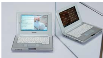
Switchable viewing-angle LCD (prototype) The content can be seen from the front, but not from the side (Reflected in a mirror)
