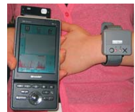
Handheld terminal capable of sending and receiving measurement information and instructions
